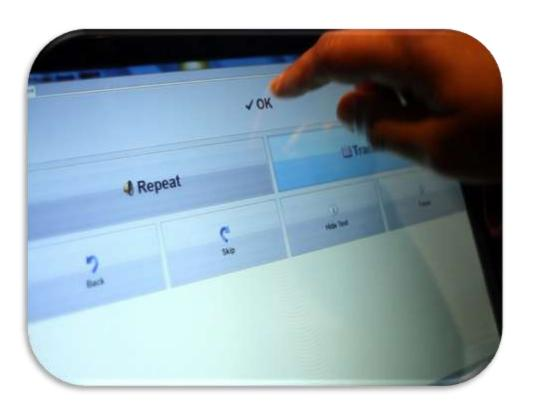
Users are supported throughout the task by a Graphical User Interface for dialogue with the system: They can request a repetition, a repetition with a particular emphasis on key words, an image or even a video!
