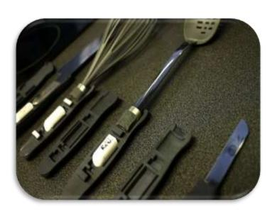
Sensors are attached to all utensils, ingredients and different parts of the kitchen
