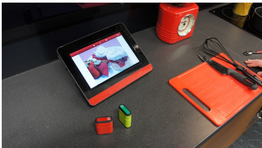
Figure 1: The touchscreen, interaction tools and some utensils with sensors which make up the portable kitchen
